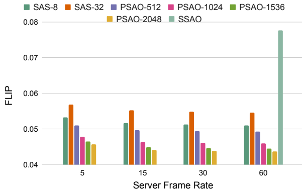
Figure 5: At varying server frame rates, PSAO outperforms SAS when averaged across all scenes. For SAS, we denote the per-patch downsampling bias factor B as SAS- B . For PSAO, we denote the number of points per unit area N as PSAO- N . Even at only 5 frames per second, PSAO can keep up with SAS, which was tuned for low server frame rate streaming of texture-space shading.
