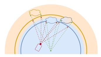
**Figure 3:** Setup with two spheres (blue, orange). The color-coded background shows the caching regions of both spheres. Clouds are colored based on their caching sphere with the right-most cloud being cached partially on both spheres.
