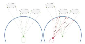
**Figure 2:** Visualization of the single spheres (blue) setup. (Left) Perfect aligned view direction and cache update direction (green arrows) producing no distortions. (Right) Camera is moved off-center resulting in differences between the view direction (red arrows) and cache update direction (green arrows) producing distortions.
