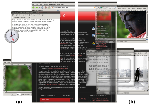
Figure 1. (a) Conventional overlapping windows occlude important information in obscured windows. To reveal this information, the user has to change the window layout manually. (b) Importance-driven compositing spatially arranges occluded windows and applies see-through compositing to maximize content visibility and interactivity.
